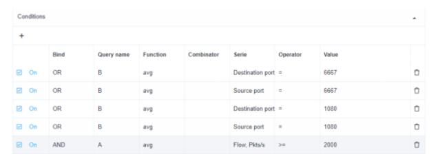
Most often, BotNet uses ports 6667 and 1080 - add each destination/source port by selecting query "B" with value "OR" and choose Flow Pcts/s equal or more than 2000.
