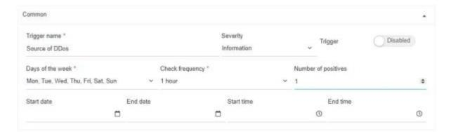
Trigger name «Source of DDoS», days of week – all, check frequency – every hour, number of positives – once, time and date of start/end - not specified.
