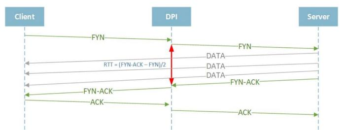
For example, this situation may occur in the case of TCP HALF CLOSED CONNECTION, i.e. when one of
