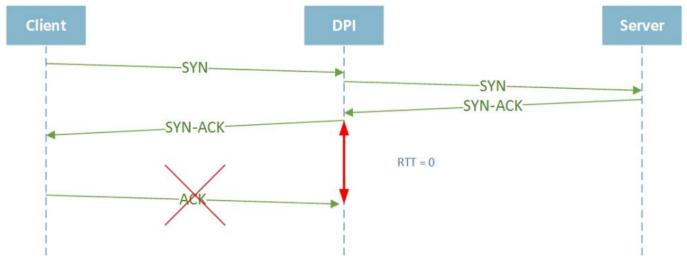
It corresponds the situation when DPI did not receive ACK sent from client to the DPI in response to received SYN/ACK. The situation can be caused by several reasons, for example, if the client physically disconnected the wire or sent RST. In all the situations mentioned above, the DPI will set "0" value in RTT from the client to the DPI for the given flow.
