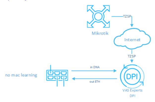
Mikrotik is able to send the subscriber traffic copy using the TZSP protocol, which is an encapsulation protocol used to wrap other protocols. To receive the traffic copy, we will use server with the Stingray Service Gateway installed (it is possible to use a dedicated server).
