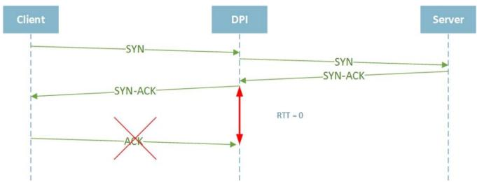
It corresponds the situation when DPI did not receive ACK sent from client to the DPI in response to received SYN/ACK. The situation can be caused by several reasons, for example, if the client physically disconnected the wire or sent RST. In all the situations mentioned above, the DPI will set "0" value in RTT from the client to the DPI for the given flow.
