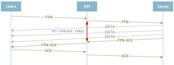
For example, this situation may occur in the case of TCP HALF CLOSED CONNECTION, i.e. when one of the connection participants terminates the data transmission, but still continues to receive the data from the remote side. In this case, the transmitting side can send FYN/ACK only after the data transfer is completed, so it will cause the significant increasing of RTT value.
