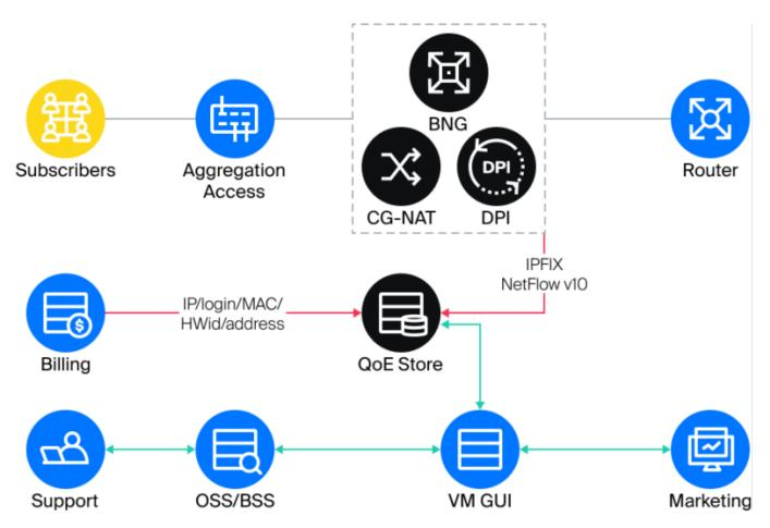
The following components are required for QoE: QoE Stor and Graphical User Interface.
