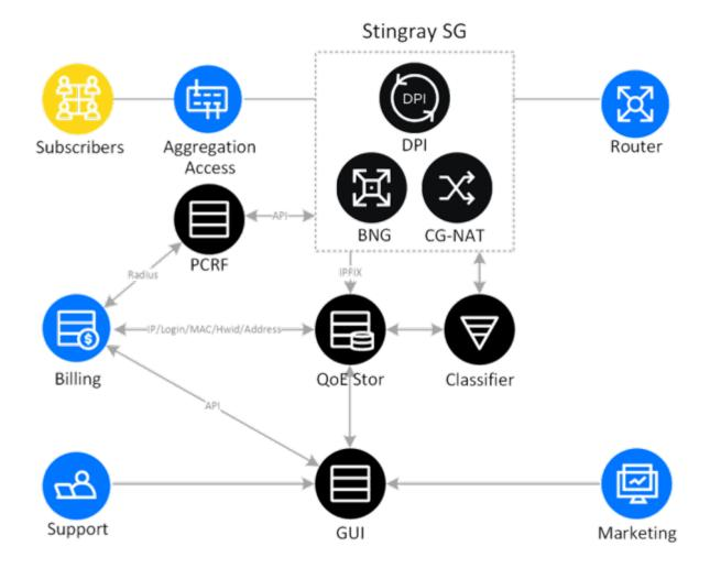
The best option is to combine CG-NAT, DPI and BNG functionality on a single device. In this way to build a flexible and easily manageable core network – this significantly reduces the TCO (Total Cost of Ownership) through compactness, high performance, uniform management and operation.
