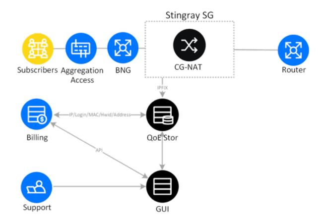
This is a classic scheme of including a CG-NAT device in the network – between the BNG and the router to provide network address translation. NAT log is transferred via IPFIX protocol (NetFlow v10) to a dedicated server or VM, where the database of this QoE Stor and GUI is installed. This solution allows efficient storage and searching of NAT logs.
