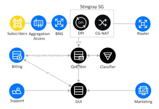
We offer to combine CG-NAT functionality with DPI on one device, not only to broadcast addresses, but also to detect and classify traffic by protocols and directions, to use common channel policing, to mark traffic, to work with statistics (Full NetFlow and Clickstream).
