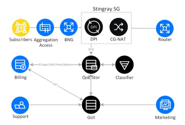
We offer to combine CG-NAT functionality with DPI on one device, not only to broadcast addresses, but also to detect and classify traffic by protocols and directions, to use common channel policing, to mark traffic, to work with statistics (Full NetFlow and Clickstream).
