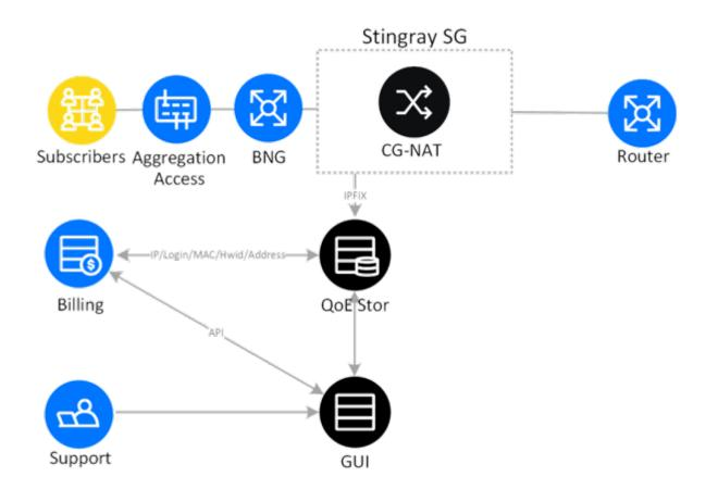
This is a classic scheme of including a CG-NAT device in the network – between the BNG and the router to provide network address translation. NAT log is transferred via IPFIX protocol (NetFlow v10) to a dedicated server or VM, where the database of this QoE Stor and GUI is installed. This solution allows efficient storage and searching of NAT logs.
