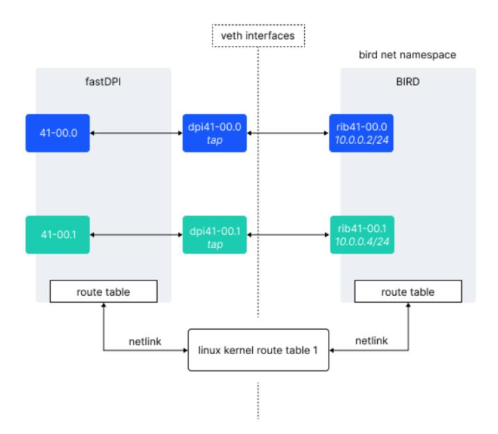
Data from the kernel route table is read (rtnetlink) in the router's RIB. RIB is a prefix tree, it is convenient to modify it by kernel route table change events (delete/add entries). But it is impossible to use RIB in routing because it does not support multithreaded access from work threads (it requires locking, which is unacceptable). Therefore, in SSG, RIB is in router thread and unavailable for worker threads.
