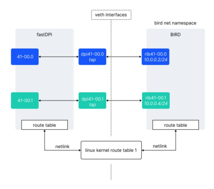
Data from the kernel route table is read (rtnetlink) in the router's RIB. RIB is a prefix tree, it is convenient to modify it by kernel route table change events (delete/add entries). But it is impossible to use RIB in routing because it does not support multithreaded access from work threads (it requires locking, which is unacceptable). Therefore, in SSG, RIB is in router thread and unavailable for worker threads.
