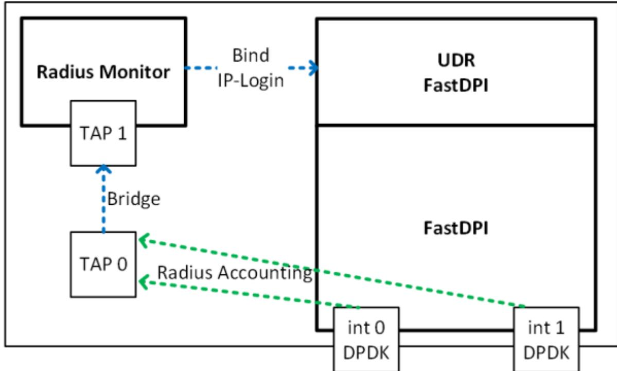
Placing Radius monitor on the same server. Bridge used.
