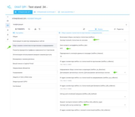
Then specify socket for fullflow receiver within "netflow\_full\_collector" parameter: "IP address of the netflow collector with full statistics (netflow\_full\_collector)". "netflow\_full\_collector\_type" should be set to "Export ipfix to udp header", whereas "netflow\_full\_port\_swap" should be empty or equals to "Keep original port numbers". See the figure below.
