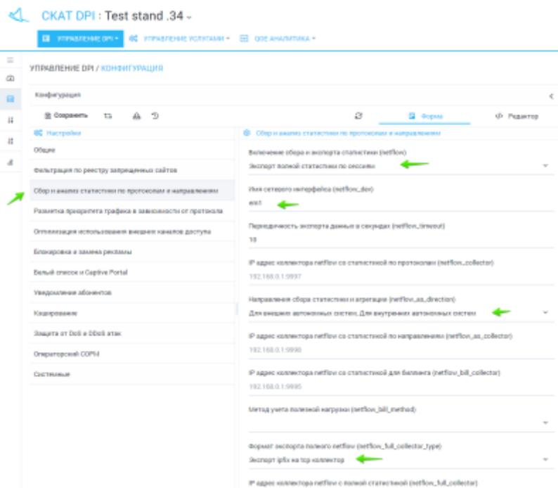
Enter the receiver's fullflow socket in the netflow\_full\_collector parameter. The
