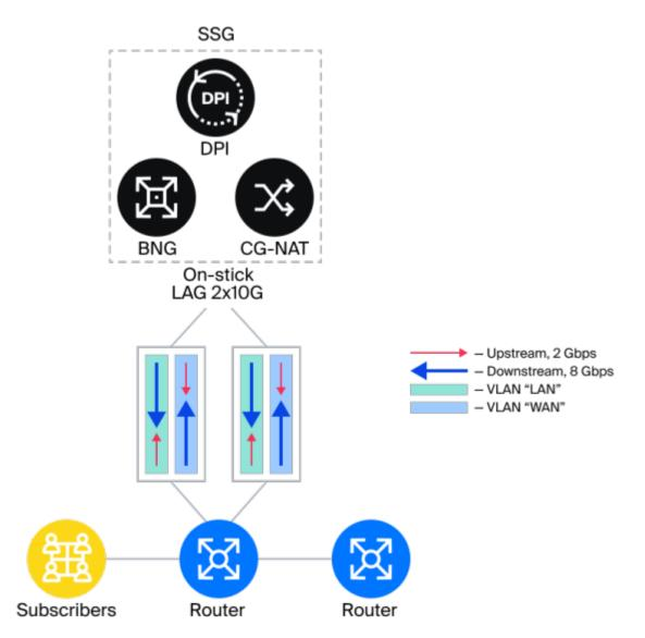
Each op-stick port is described in a specific way: first the base physical port is described using dpdk\_device, then the virtual ports based on the base port are described. Description of the base devices:
