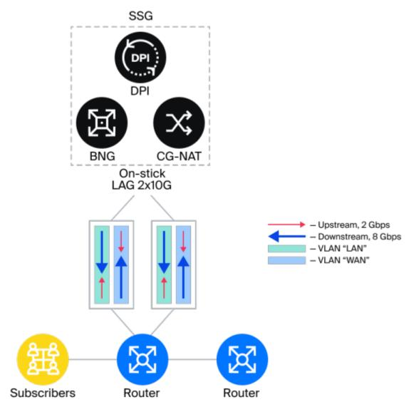
Each op-stick port is described in a specific way: first the base physical port is described using dpdk\_device, then the virtual ports based on the base port are described. Description of the base device:
