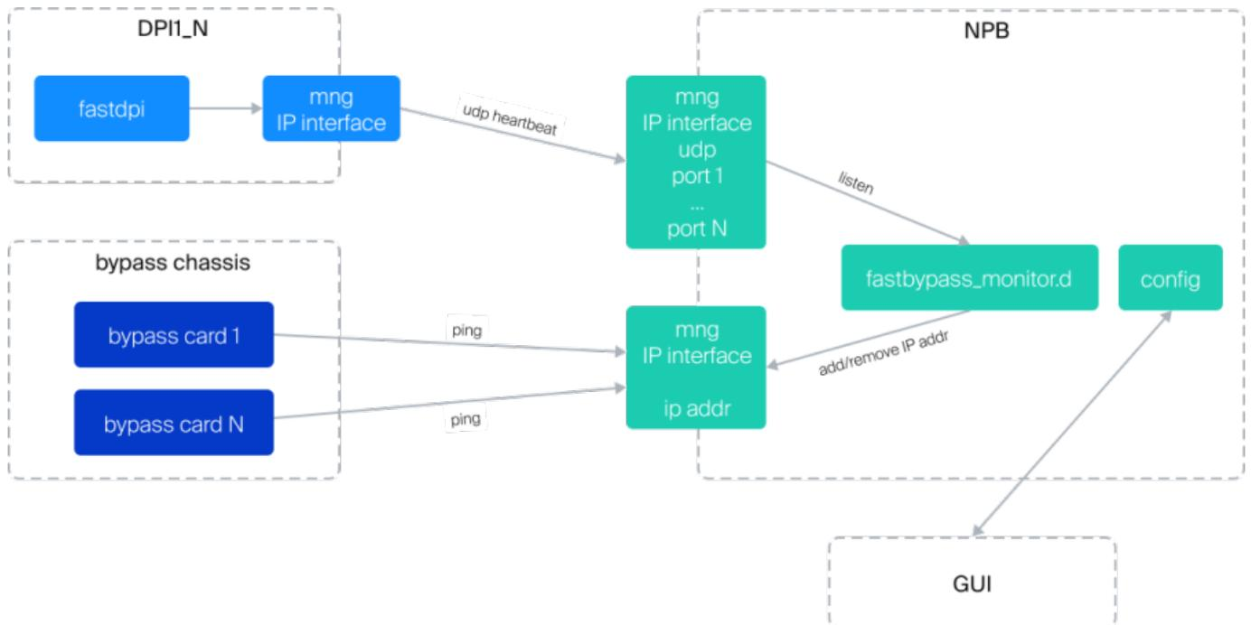
If there is a software failure on DPI, the NPB removes the DPI from the stack and redistributes the load among the remaining DPIS.
