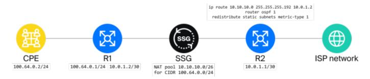
On router R2, it will be necessary to configure the route to the NAT pool. For Cisco-like CLI, the configuration will look like this:
