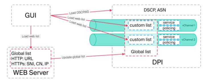
A dedicated web server is used for centralized Global Lists loading onto DPI. FilterUI exports lists to this server in a prepared format for DPI. Each DPI downloads these lists and applies them according to rules. Additionally, FilterUI exports unique rules for each DPI. If necessary, these lists are merged and applied to a channel or subscriber.
