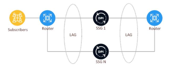
Balancing in the LAG is necessary to ensure symmetrical traffic through each SSG device.
