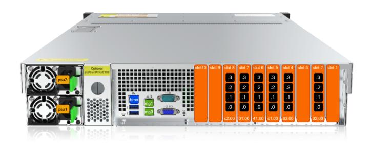
Cards with 10/25/40/100 network ports are placed in slots 1-10 Each slot has a unique PCle bus identifier, e.g. 02:00. Each port has a unique identifier on the card, e.g. 02:00.0, 02:00.1, 02:00.2, 02:00.3.
