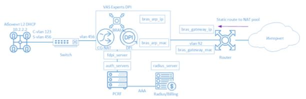
BRAS DHCP L2 mode means that the subscriber recieves an IP-address via DHCP Proxy and proceeds to AAA in the Billing system. Then the subscriber is terminated by Stingray Service Gateway(SSG) and transferred to border equipment.
