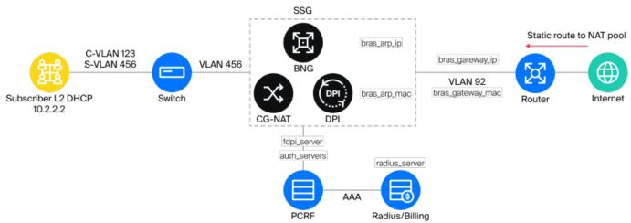
BRAS DHCP L2 mode means that the subscriber recieves an IP-address via DHCP Proxy and proceeds to AAA in the Billing system. Then the subscriber is terminated by Stingray Service Gateway(SSG) and transferred to border equipment.
