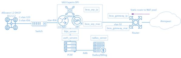
BNG/BRAS DHCP L2 means that Stingray Service Gateway (SSG) acts as a DHCP Relay. The subscriber is authorized by the allocated IP-address after successful session initiation. Then the IP-address is terminated with a DPI and goes to the border.
